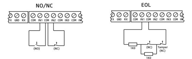
When connecting the inputs of Pager8, NO, NC and EOL wiring can be used depending on the application. In the figures above, you will find examples for each of the three. In the first figure, IN1 is shown as normally open (NO), and IN2 is normally closed (NC). The second figure shows the EOL connection of IN1.
