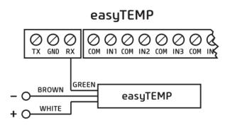
The easyTEMP's data wire (green) must be connected to the serial port input of the Pager8 (marked with RX on the connector), and the ground (-) of the easyTEMP and Pager8 must be equipotential. (It is recommended to connect both devices to the same power source.)
