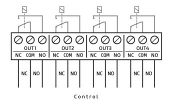
There are two ways to connect the outputs according to usage. If you want to use the output in NC (normally closed) mode, use the NC and adjacent COM connectors of the corresponding relay as shown in the picture. For NO (normally open) mode use the NO and COM connectors.
